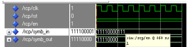
Fig. 34 removing cyclic prefix emulation results
