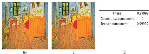
Fig 6:a) Watermarked Image with white noise, b) Watermarked image after reducing the noise, c) correlation between the watermarked image after extraction of the watermark and the original image as well as the correlation between the two components (u and v only).
