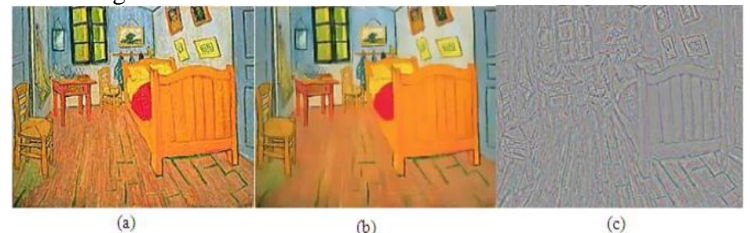
fig 1: Color decomposition: (a) initial image f , (b) cartoon component u , (c) texture component v .
