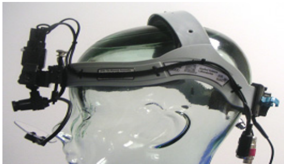
Fig. 1: Eye Tracker ASL6000 Model
