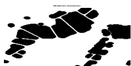
Fig.13 Shows 3x times dilation followed by 3x times erosion (4x4 structural elements)
