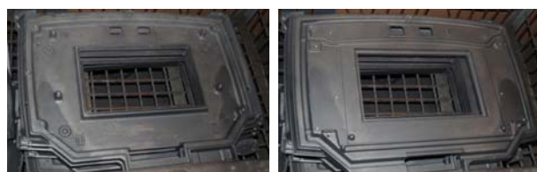
Fig. 1.a. Markers cast on corners on parts b. parts turned around (Note: Variation in dark and light regions on the part due to changeover of molten iron batch)
