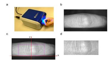
Fig-1: a)Image acquisition device is being used to collect FKP samples b)Sample FKP image c)ROI coordinate system, where the rectangle indicates the area d)Extracted ROI
