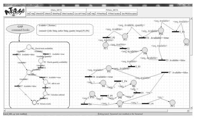
Fig. 13 The generated equivalent PrT-Net model of "Command-books"
