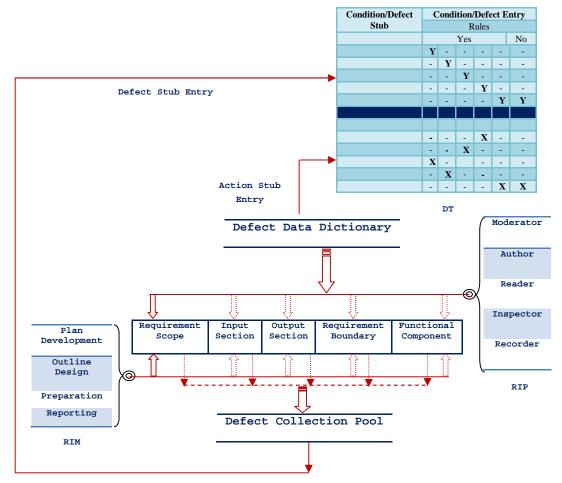
Proposed Framework to Requirement Defect Identification
