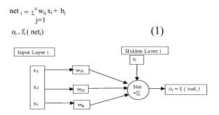
Figure 1: Model of a perceptron
