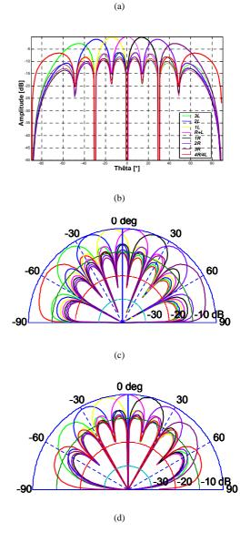
Fig. 5 Performance of the Butler matrix 8x8 standard (a),(b): Simulated radiation pattern in Cartesian coordinates respectively 3 dB/90° couplers and 3 dB/180° couplers (c),(d) : Simulated radiation pattern in polar coordinates3 dB/90° couplers and 3 dB/180°
