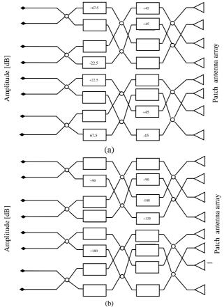
Fig. 4 Functional schematic Butler matrix (a):with 3 dB/90 $^{\circ}$  couplers (b) :with 3 dB/180 $^{\circ}$  couplers
