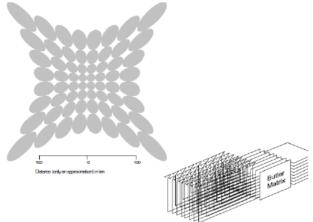
Fig .6 A two-dimensional Butler matrix producing orthogonal beams[7]
