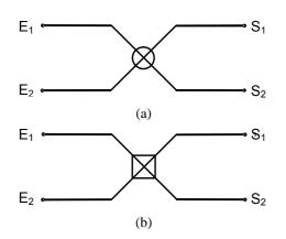
Fig. 1 Functional representation (a) 3 dB coupler 90 °,(b) 180 ° 3dB couplers.
