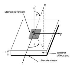
Fig. 2 Microstrip patch antenna
