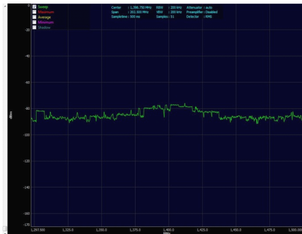
Figure 4: Power level in dBm versus frequency (1.3-1.5GHz)
