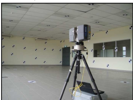
Fig. 8: Self-calibration for the Faro Photo 120 scanner.
