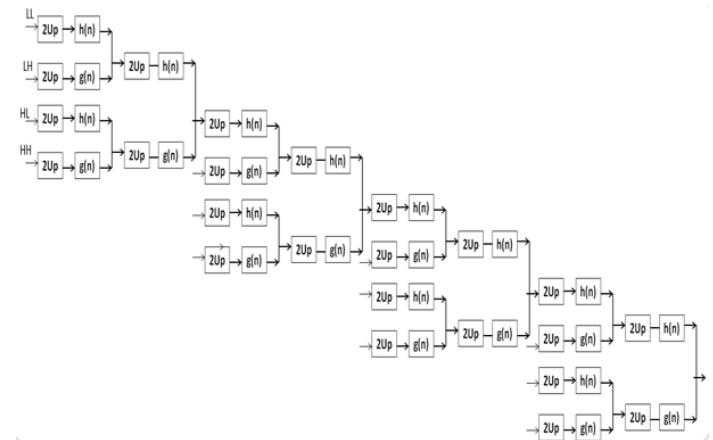
Fig. 28 2D Image Reconstruction at stage-4
