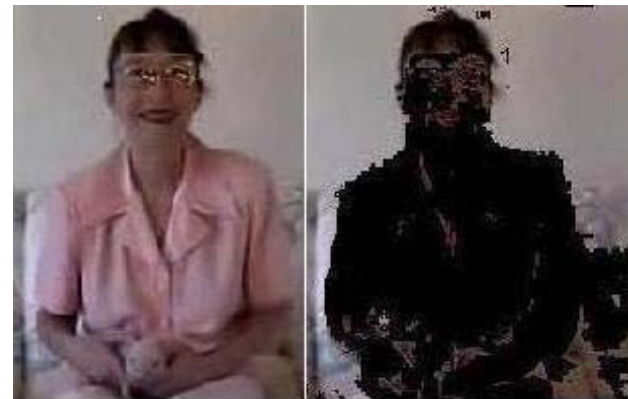
(a) Skin detection example on a frame from Video 12. Black shows skin.
